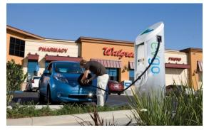
stations can add up to 30 miles to the range of an electric car in 10 minutes of charging. The Level 2 charge can tack on 25 more miles to the overall range on an hour's worth of charging.
