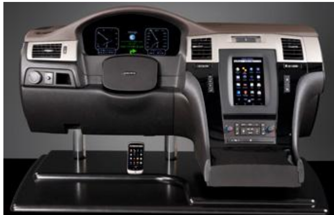
Smart phone screen replicated on center stack in Delphi's dashboard concept.
